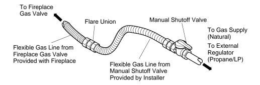
Figure 36 - Attaching Flexible Gas Lines Together
